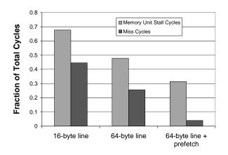
Figure 8: Average fraction of simulated cycles for AUTCOR, CONVEN, IP\_CHECKSUM, and IMGBLEND spent waiting in the vector memory unit in total or exclusively servicing a miss for a 16-lane full memory crossbar VESPA processor when cache lines are widened to 64B and prefetching is enabled for the next 15 cache lines.
