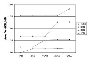
Figure 3: System area for different cache depths and cache line sizes normalized against the system with 4KB cache with 16B line size. Each line in the graph depicts a different cache line size.
