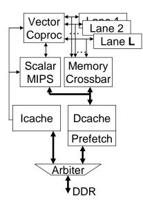
Figure 1: VESPA processor block diagram.
