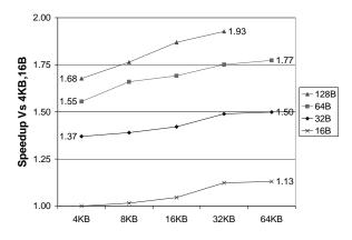
Figure 2: Wall clock speedup attained for different cache depths and cache line sizes over the 4KB cache with 16B line size. Each line in the graph depicts a different cache line size.
