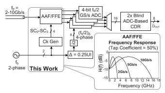
Fig. 2. Proposed analog front-end for a 2x blind ADC-Based RX.
