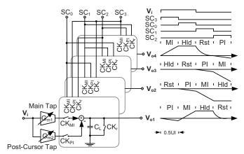
Fig. 3. The overall AAF/FFE system block diagram.
