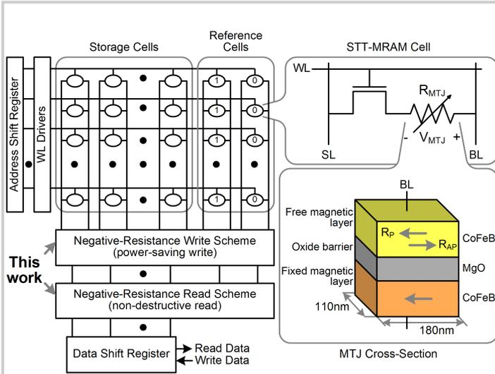
Figure 14.1.1: Simplified block diagram of STT-MRAM array.
