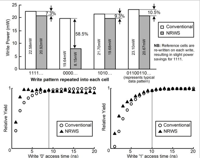
Figure 14.1.6: Measured write power consumption and access time.
