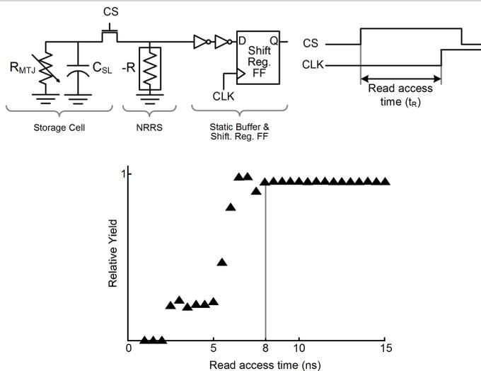
Figure 14.1.5: Measurement setup and measured NRRS read access time.
