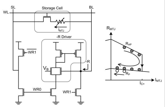
Figure 14.1.4: Negative-resistance write scheme (NRWS) implementation.
