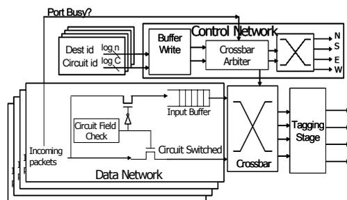
Fig. 2. Switch Design
