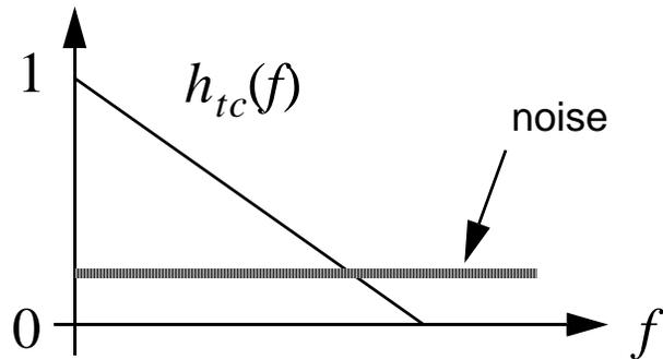
Transmit filter, channel and noise
