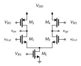
Based on a small-signal analysis approach, find the input offset of the amplifier (the sign of the offset is unimportant).
