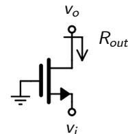
Accurate:  $R_{out} = r_o + (1 + g_m r_o)R_S$
