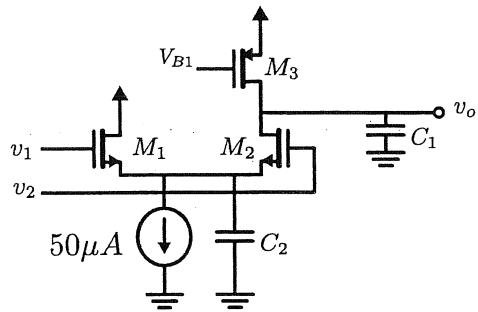
$$\begin{aligned}V_{ov1} &= V_{ov2} = 0.1V \\V_{ov3} &= 0.4V \\ \text{All } r_o &= 100k \\ C_1 &= 1pF \\ C_2 &= 2pF\end{aligned}$$
