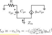
$$L_O \equiv -v_r/v_t = -\left(\frac{-1/sC_{gs}}{1/sC_{gs}+R}\right)g_m\left(\frac{1+sC_{gs}R}{sC_{gs}}\right) = \frac{g_m}{sC_{gs}}$$
