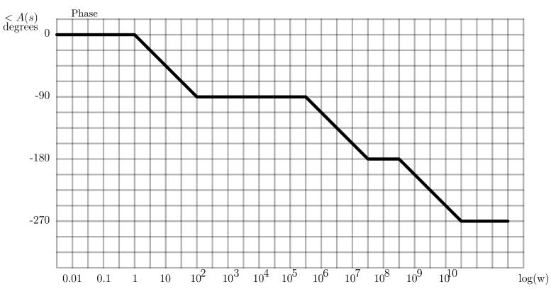
(b) Estimate the phase-margin (PM) if the above opamp is used to create a gain of +3 using 2 resistors (a non-inverting configuration) (Hint: Note that the unity-gain frequency is much greater than  $\omega_{p1}$  and much less than  $\omega_{p3}$ .)
