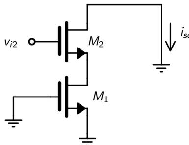
$$G_{Mb} = (-g_{m2} * r_{o2}) / (r_{o2} + (1 + g_{m2} * r_{o2}) * r_{o1}) = -(500e-6) * (10e3) / ((10e3) + (1 + (500e-6) * (10e3)) * (20e3)) = -38.46e-6$$
