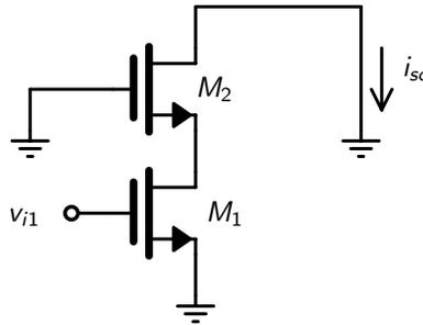
Define  $R_{S2}$  to be the impedance looking up into the source of  $M_2$
