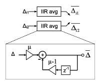
Fig. 20. Detail of IIR filter blocks used in "estimate error" block of Fig. 21.
