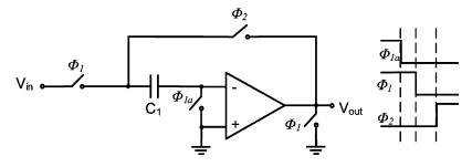
Fig. 16. Sample and hold topology (implemented fully differentially in this work).
