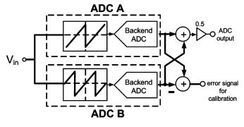
Fig. 4. Example split-ADC topology.
