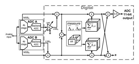
Fig. 14. Full ADC topology of this work.
