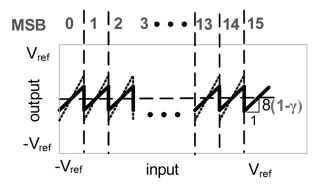
Fig. 8. Residue transfer curve showing impact of gain errors.
