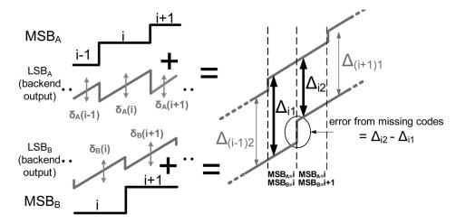
Fig. 12. Transfer curves of key ADC outputs with gain, DAC errors included.
