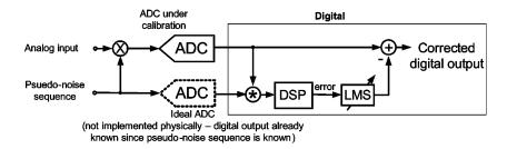
Fig. 3. Principle of background calibration.
