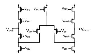
Fig. 19. Opamp used in first stage MDAC.
