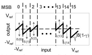
Fig. 9. Residue transfer curve showing impact of DAC and gain errors.
