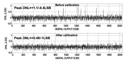
Fig. 24. DNL before and after calibration.
