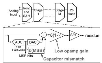
Fig. 5. Pipeline topology, first stage shown in detail including error sources.
