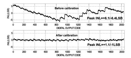
Fig. 23. INL before and after calibration.
