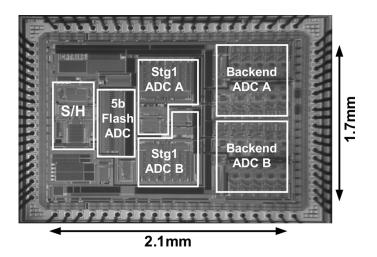
Fig. 22. Micrograph of fabricated IC in 1.8 V 0.18  $\mu\rm{m}$  CMOS.
