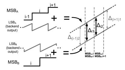
Fig. 11. Transfer curves of first stage (MSB), backend ADC (LSB) and total ADC outputs from each split ADC with no errors.
