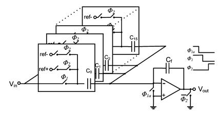
Fig. 6. Example implementation of 4-bit MDAC (shown single-ended, implemented differentially in practice).
