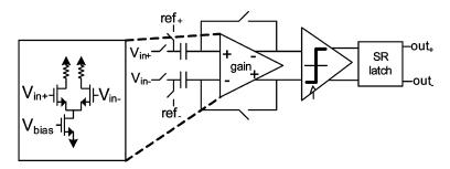
Fig. 17. Comparator topology used in 5-bit Flash sub-ADC.
