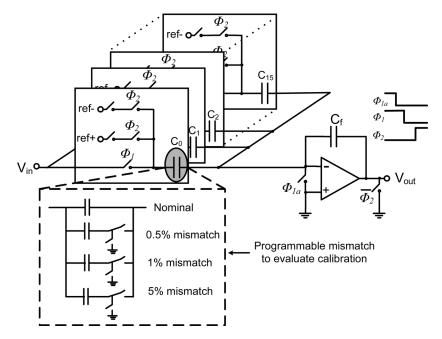
Fig. 18. Topology of first stage MDAC (implemented fully differentially in this work).
