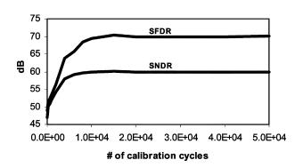
Fig. 27. ADC SNDR, SFDR improvement with number of calibration cycles.
