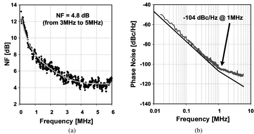
Fig. 13. (a) Noise figure and (b) phase noise measurements.
