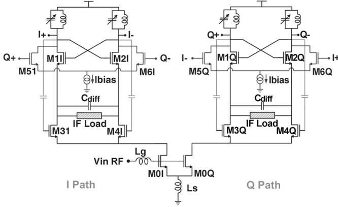
Fig. 4. LNA's low-frequency degeneration for LMV cell phase noise reduction.
