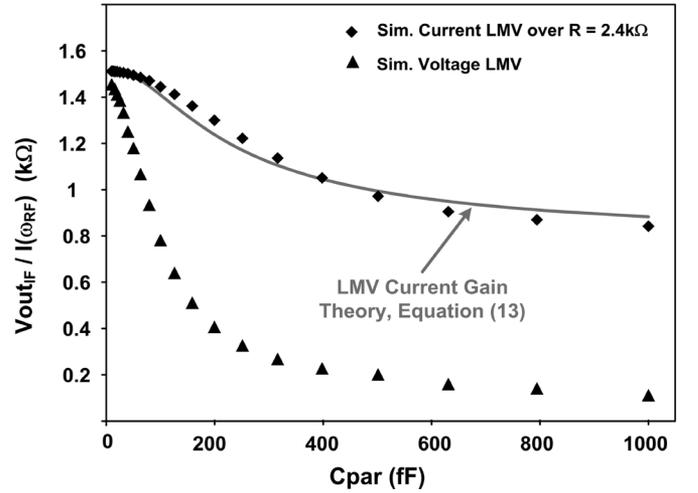
Fig. 9. Simulations of current-mode and voltage-mode gain as function of  $C_{par}$ .
