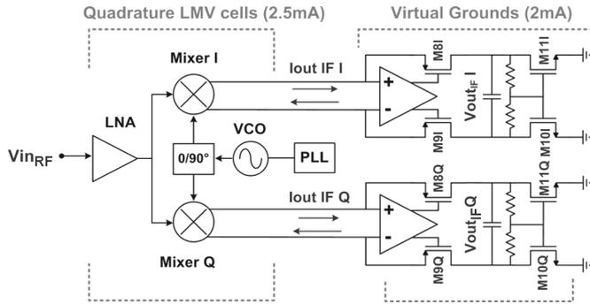
Fig. 10. Complete RF front-end based on low-IF architecture for GPS receiver.
