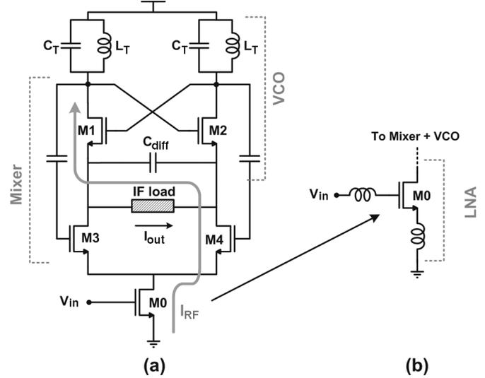
Fig. 3. Double switching pair self-oscillating mixer and LMV.
