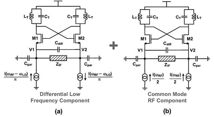
Fig. 7. Loss mechanisms. (a) Low-frequency components. (b) RF components.
