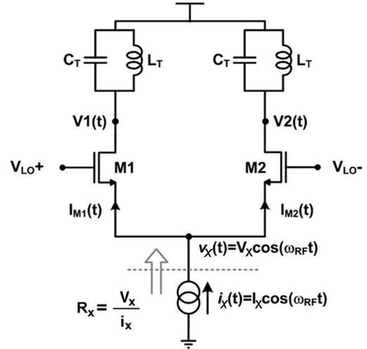
Fig. 16. Circuit for the calculus of RF impedance at the M1–M2 sources.
