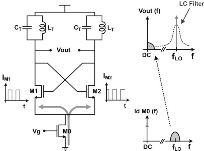
Fig. 1. LC tank oscillator as a mixer.
