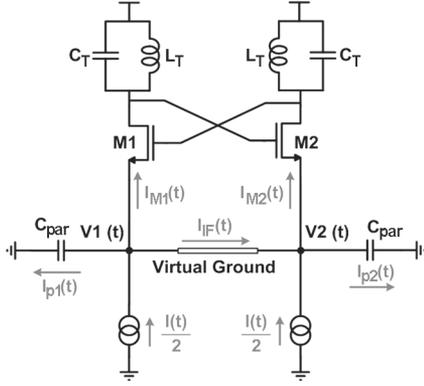
Fig. 8. Current-mode LMV cell.
