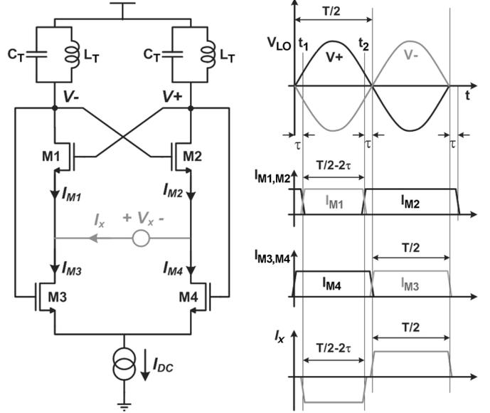
Fig. 6. Voltage gain upper bound. (a) Circuit for the calculus. (b) Currents waveforms.
