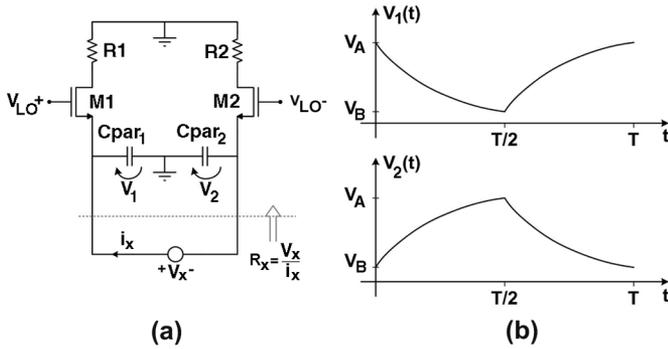
Fig. 14. Circuit for switched-impedance calculation and voltage waveforms.
