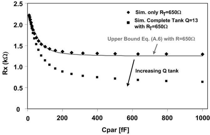
Fig. 15. Switched-impedance losses versus  $C_{\text{par}}$ .
