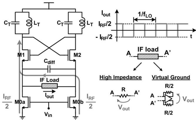
Fig. 2. Bias splitting self-oscillating mixer.
