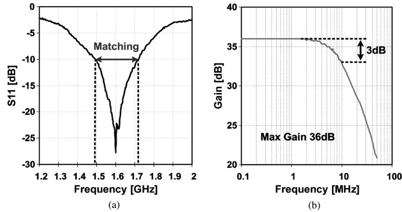
Fig. 12. (a) Input matching and (b) in-band gain measurements.
