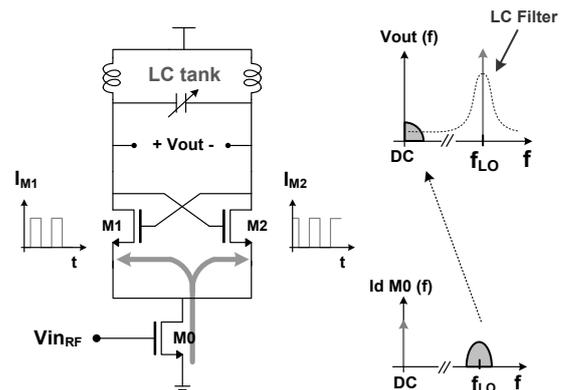
Fig. 1. LC tank oscillator as a mixer.
