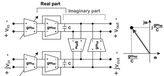
Fig. 8 Gm-C complex pole synthesis
