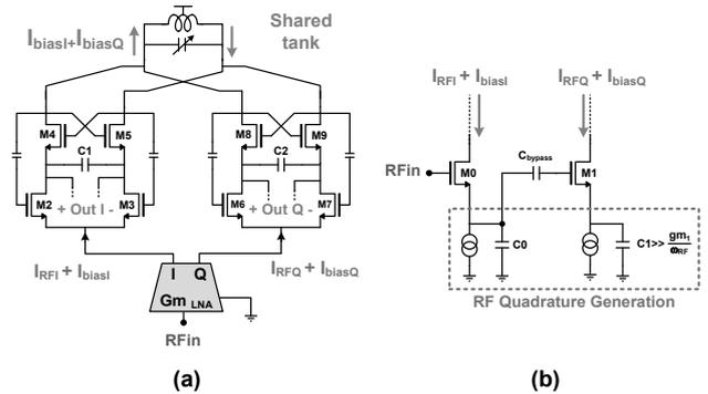
Fig. 4. Quadrature generation on the RF signal path: (a) single coil quadrature LMV cell, (b) stacked quadrature LNA.
