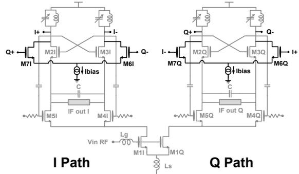
Fig. 3. LO Quadrature generation: Cross Coupled LMV scheme.
