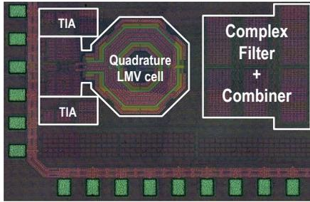
Fig. 7 ZigBee receiver scheme and chip micrograph
