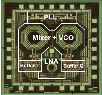
Fig. 5 GPS prototype circuits and chip micrograph.
