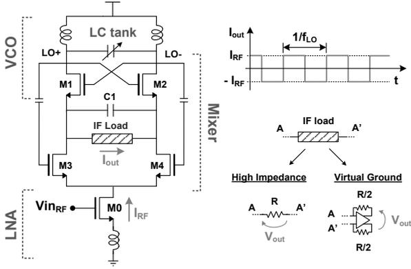
Fig. 2. The LNA-Mixer-VCO cell (bias not shown)
