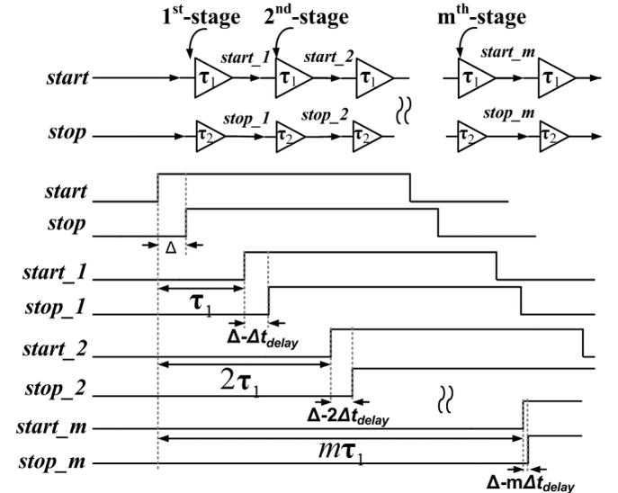
Fig. 3. Signal evolution in a Vernier TDC.
