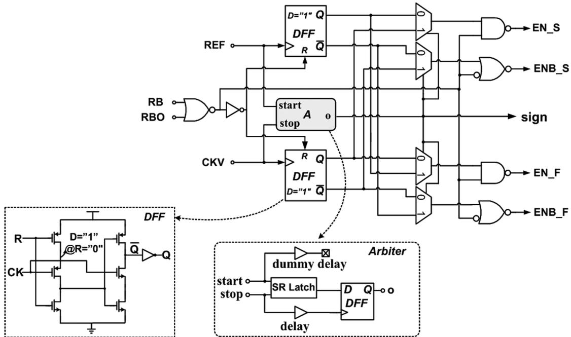
Fig. 9. Adaptive phase-frequency detector.
