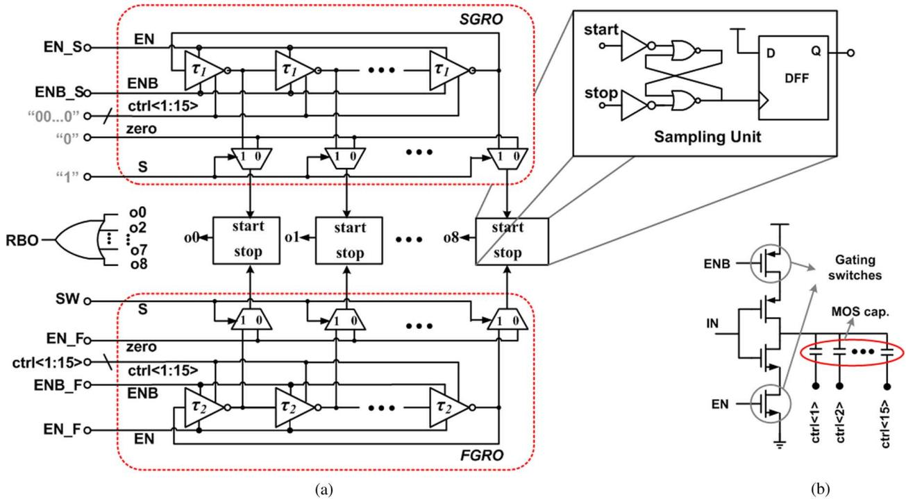
Fig. 6. Vernier GRO (a) core part, (b) gated inverter (cell) with capacitive delay control.
