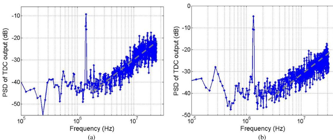
Fig. 13. Measured TDC output PSD with sinusoidal delay input (a) Vernier resolution = 15 ps@50 MHz, (b) Vernier resolution = 6 ps@62.5 MHz.
