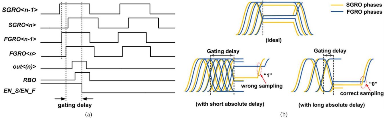
Fig. 7. Gating delay: (a) waveform illustration, (b) effects for short and long absolute delay.
