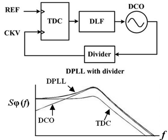
Fig. 1. top: DPLL with TDC; bottom: main noise contributions at DPLL output.
