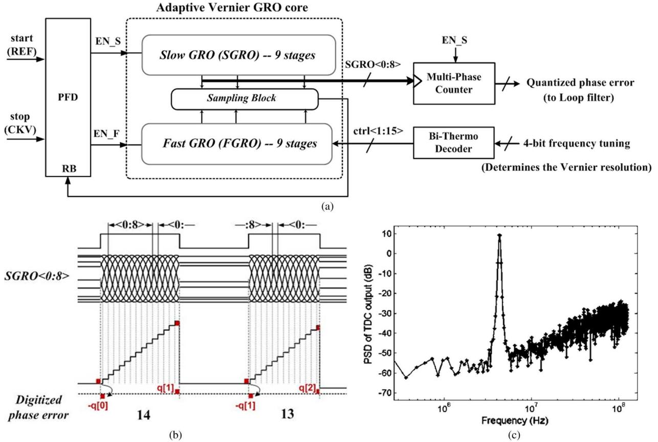
Fig. 4. The proposed TDC: (a) block diagram, (b) multi-phase counting and noise-residue accumulation, (c) first-order quantization noise shaping in frequency.
