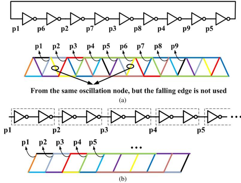
Fig. 5. The phase sequence concerning only rising edges (a) in a ring oscillator; (b) in a delay line.
