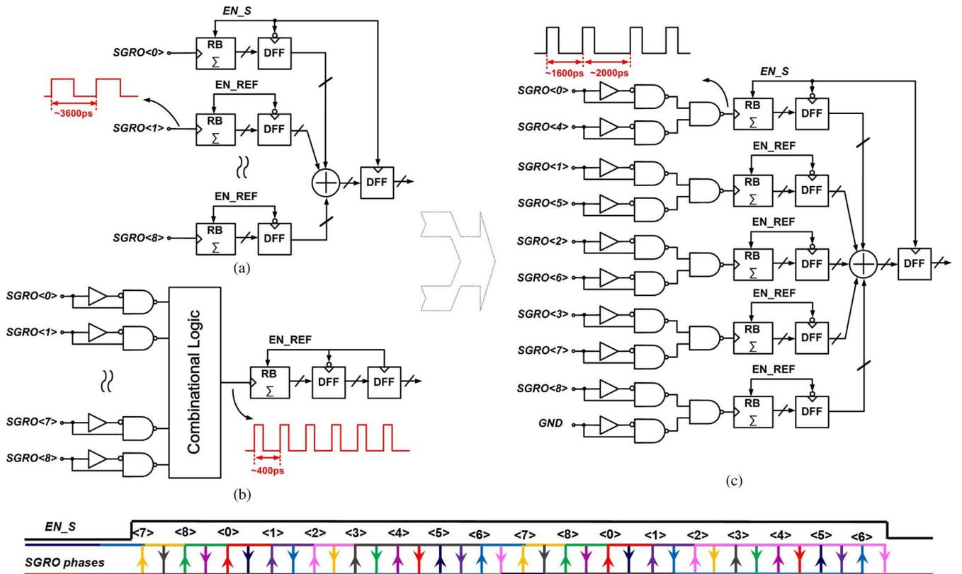
Fig. 10. Multi-phase counter with (a) an individual accumulator for each SGRO phase, (b) only one accumulator with all SGRO phases combined to a single one, (c) proposed trade-off solution.
