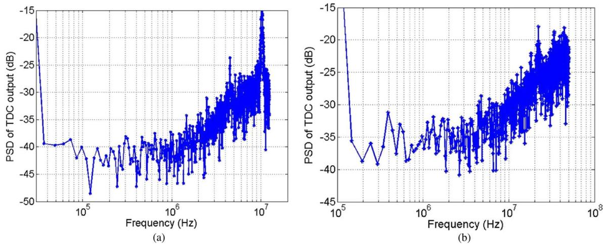
Fig. 12. Measured TDC output PSD with dc delay input of 20 ps: (a) Vernier resolution of 5.8 ps @25 MHz, (b) Vernier resolution of 6.5 ps @100 MHz.
