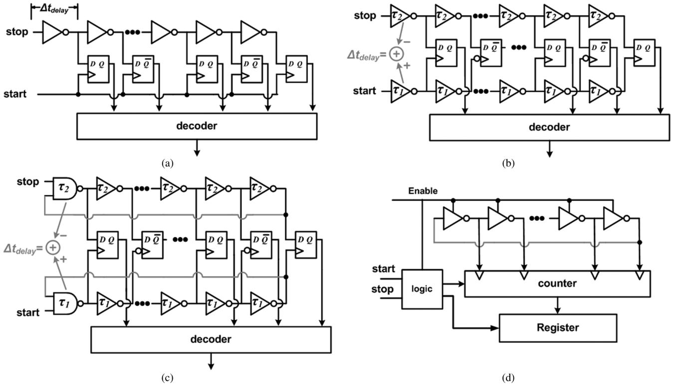
Fig. 2. Different TDC architectures: (a) basic delay-line TDC, (b) Vernier TDC [11], (c) Vernier ring-oscillator TDC [14], (d) gated-ring-oscillator TDC [15].
