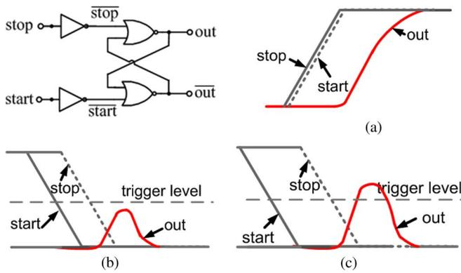
Fig. 8. SR latch: (a) correct sampling when *stop* catches up with *start*, (b) acceptable *start-stop* delay.
