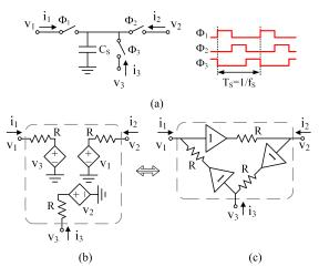
Fig. 16. a) A three-phase switched-capacitor topology, and b,c) its continuous-time model.
