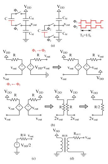
Fig. 6. a) Switched-capacitor DC/DC voltage converter, b) its simplified continuous-time model, c) Thévenin equivalent of  $v_{out}$  obtained with the continuous-time model, d) conventionally used switched-capacitor converter transformer model.
