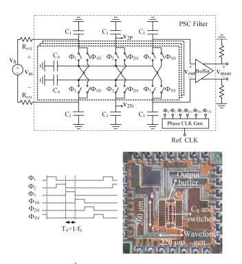
Fig. 12. Fabricated 3<sup>rd</sup>-order low-pass PSC low-pass filter schematic, timing diagram, and chip photo.
