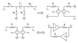
Fig. 4. A common non-grounded switched-capacitor structure modeling.
