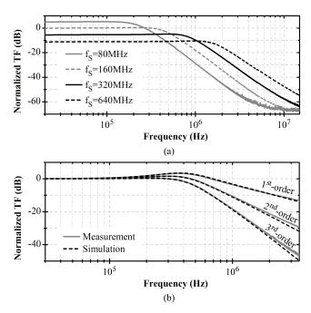
Fig. 14. Measured low-pass PSC filter a) output response for changing sampling frequencies,  $f_S$ , and b)  $1^{st}$ ,  $2^{nd}$ , and  $3^{rd}$ -order output nodes for  $f_s = 160$  MHz.
