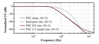
Fig. 13. Transfer functions of the simulated and measured 3<sup>rd</sup>-order low-pass PSC filter and the simulated 7<sup>th</sup>-order all real pole filter.
