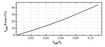
Fig. 9. Error in the 3dB cut-off frequency calculation of a 1<sup>st</sup>-order PSC filter using the continuous-time model.
