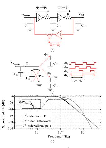
Fig. 11. a) The continuous-time model of the  $3^{rd}$ -order filter with complexconjugate poles, b) an example PSC implementation, and b) its transfer function compared with the same order Butterworth and the  $7^{th}$ -order real pole filter having the same 1 dB droop frequency.
