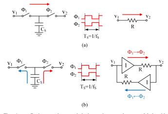
Fig. 1. Basic two-phase switched-capacitor topology modeled with a) traditional equivalent resistance, and b) two buffer + equivalent resistance branches.
