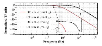
Fig. 8. 1<sup>st</sup>-order PSC filter simulated discrete-time implementation and continuous-time model frequency responses for  $C_I/C_S = 40$  and  $C_I/C_S = 4$ .
