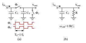
Fig. 7. a) 1<sup>st</sup>-order PSC filter and b) its continuous-time model with the traditional equivalent resistance approach.
