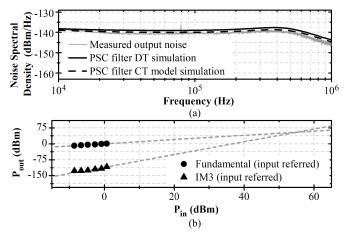
Fig. 15. a) Measured output noise spectral density over the filter bandwidth and b) out-of-band IIP3 measurements of the PSC filter with two tones.
