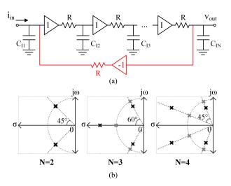
Fig. 10. a) Low-pass PSC filter with complex conjugate poles, and b) the pole locations of the  $2^{nd}$ ,  $3^{rd}$ , and  $4^{th}$  order filters, where the gray markers shows the same order Butterworth pole locations having the same 1 dB cut-off frequency.
