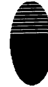
Image 3. Sampled edge points of a segment of an ellipse. White lines are used to indicate the sampled edge points.
