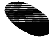
Image 6. Sampled edge points of a segment of an ellipse. White lines are used to indicate the sampled edge points.
