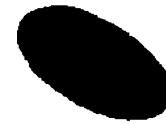
Image 4. An imaged ellipse. A binary image of an elliptical shape obtained by thresholding a grey-level image.
