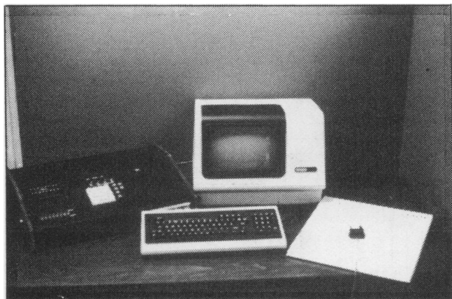
Figure 8. Input transducers for stand-alone prototype, including microprocessor-based controller. The controller is seen to the left, the CRT and keyboard in the center, and digitizing tablet to the right.
