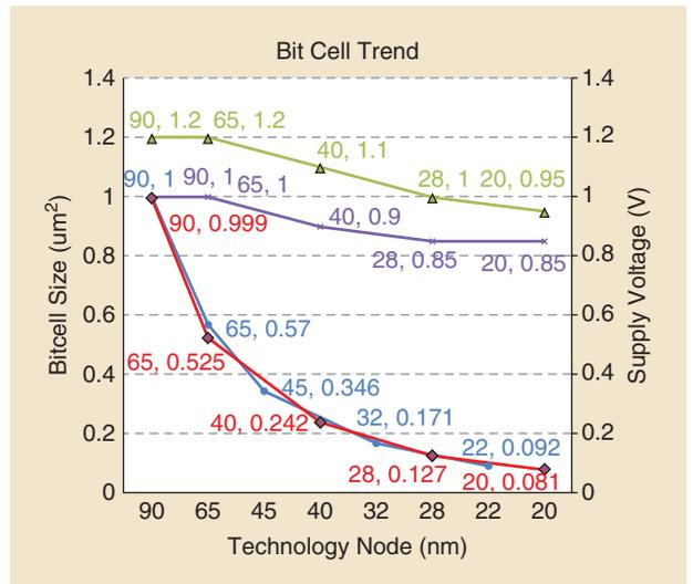
FIGURE 12: SRAM bit-cell size and supply scaling range from major semiconductor manufacturers.
