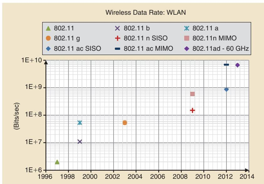
FIGURE 21: Data rate for wireless connectivity standards (802.11x).
