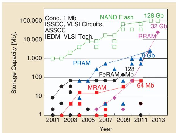
FIGURE 15: Memory capacity of emerging nonvolatile memories.
