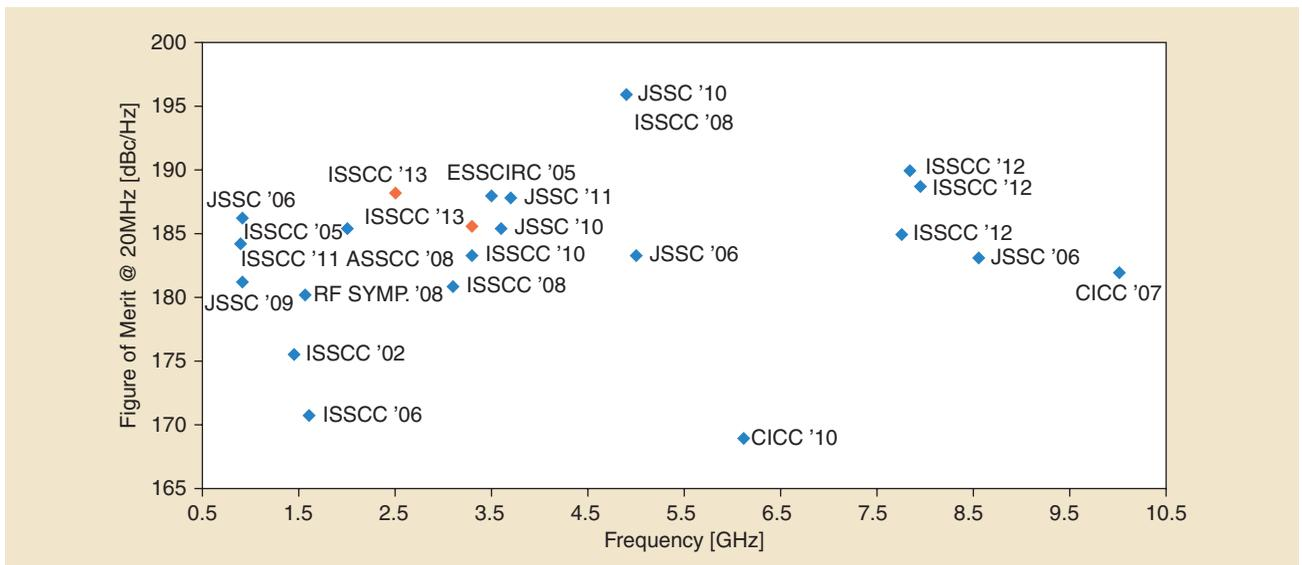
**FIGURE 19:** Phase-noise FoM at 20-MHz offset frequency versus oscillation frequency.
