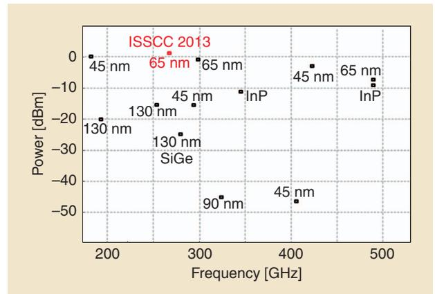
**FIGURE 18:** Output power versus frequency for mm-wave and sub-mm-wave sources.
