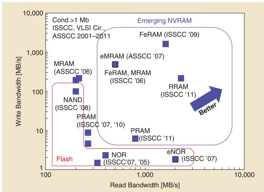
FIGURE 14: Read and write bandwidths comparison of nonvolatile memories.
