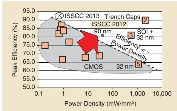
**FIGURE 1:** The development of integrated power conversion: each year, more and more is integrated in standard CMOS technologies, optimizing efficiency versus power density. At ISSCC 2013, these trends are evident in a shift to higher performance, as shown by the arrow directed to the upper right. (Adapted courtesy of ISSCC 2012 Paper 5.4.)
