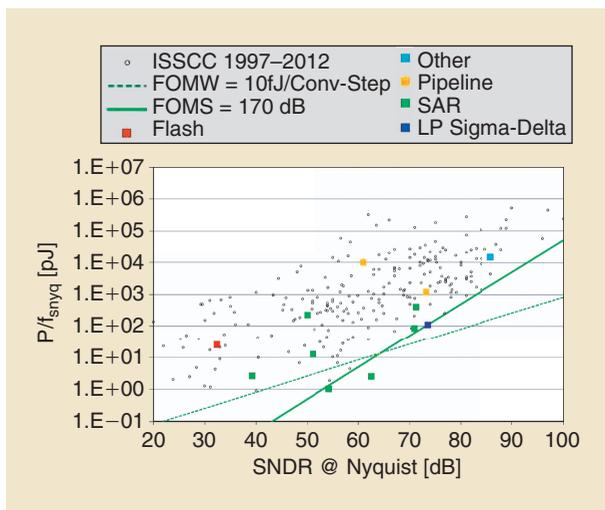
**FIGURE 2:** Power efficiency versus SNDR (highlighting ISSCC 2013 results).
