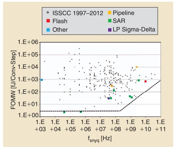
**FIGURE 3:** FoM (energy per conversion step) versus Nyquist bandwidth for various converter.
