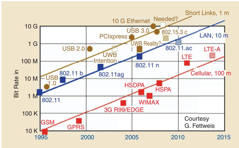
**FIGURE 6:** Wireless and wired data rates over time.
