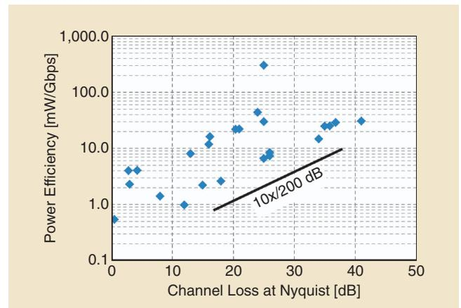
FIGURE 24: Wireline transceiver power efficiency versus channel loss.
