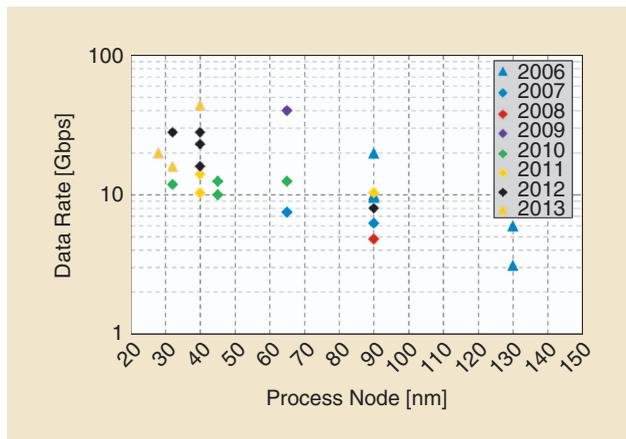
FIGURE 23: Wireline data rate versus process feature size and year.
