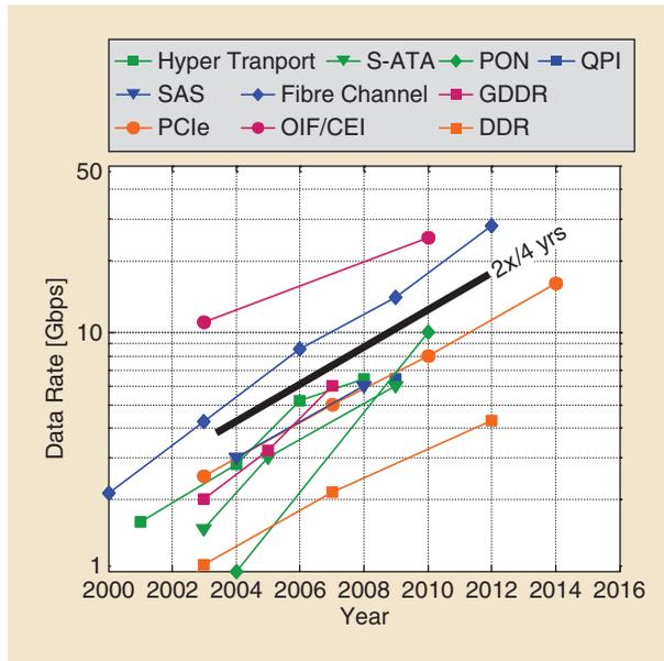
FIGURE 22: Per-pin data rate versus year for a variety of common wireline I/O standards.
