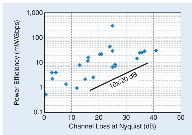
FIGURE 24: Wireline transceiver power efficiency versus channel loss.
