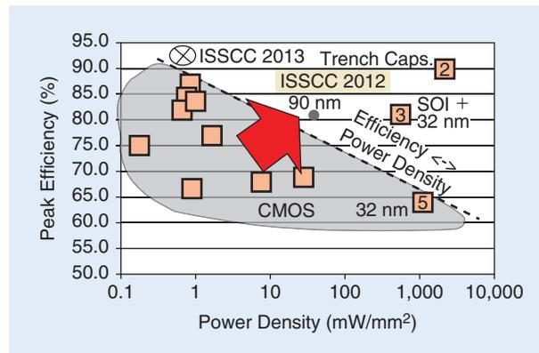
**FIGURE 1:** The development of integrated power conversion: Each year, more and more are integrated in standard CMOS technologies, optimizing efficiency versus power density. At ISSCC 2013, these trends are evident in a shift to higher performance, as shown by the arrow directed to the upper right. (Adapted, courtesy of ISSCC 2012 Paper 5.4.)
