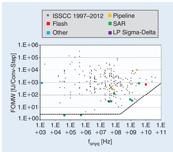
**FIGURE 3:** FoM (energy per conversion step) versus Nyquist bandwidth for various converters.
