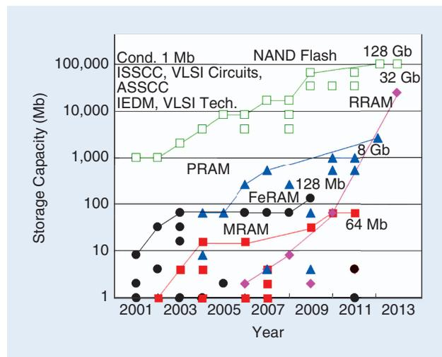
**FIGURE 15:** Memory capacity of emerging nonvolatile memories.
