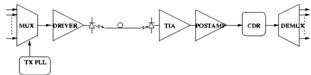
Fig.1: Typical PHY block diagram for 10 Gb/s and 40Gb/s fiber systems.
