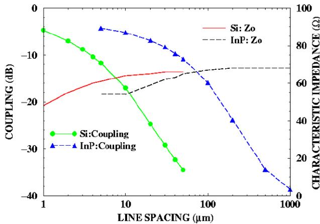
**Fig.8:** Coupling and characteristic impedance of two adjacent, infinitely long, microstrip lines on Si and InP substrates as a function of the spacing between lines.
