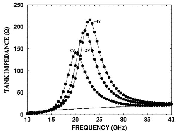
Fig.10: Measured impedance of a 20GHz VCO L-C-varactor tank fabricated in a SiGe HBT process as a function of frequency and varactor voltage [15].
