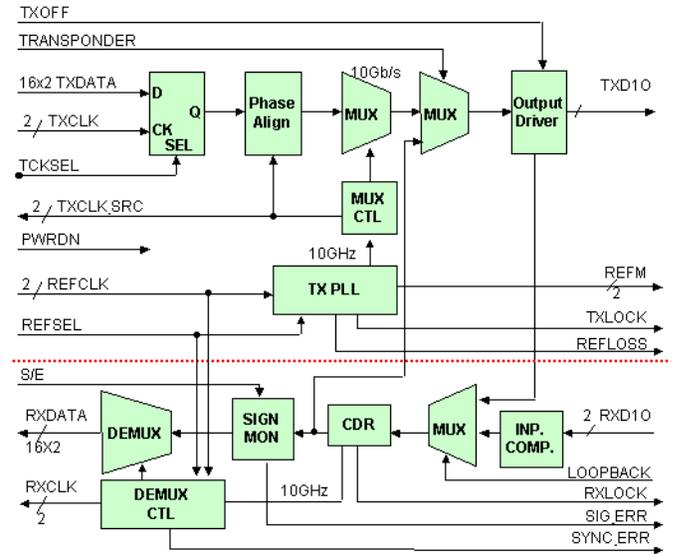
Fig.12: Block diagram of a 10Gb/s SERDES featuring 16:1 MUX/DEMUX, Clock Generation Unit, CDR, output driver with wave shape control.
