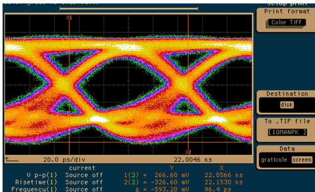
Fig.14: b) Measured 10.3Gb/s eye-diagram at the transmitter output with negative peaking only.
