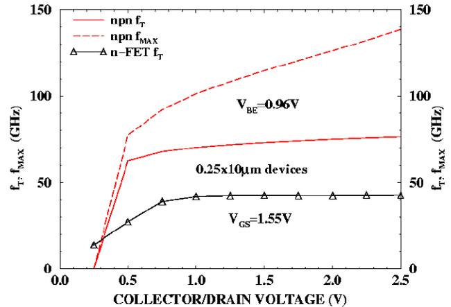
Fig.4:  $0.25 \times 10 \mu\text{m}^2$  npn  $f_T$  and  $f_{MAX}$  characteristics as a function of the collector-emitter voltage,  $V_{CE}$ . For comparison, the  $V_{DS}$  dependence of an  $10 \times 0.25 \mu\text{m} \times 10 \mu\text{m}$  n-channel MOSFET is also shown.
