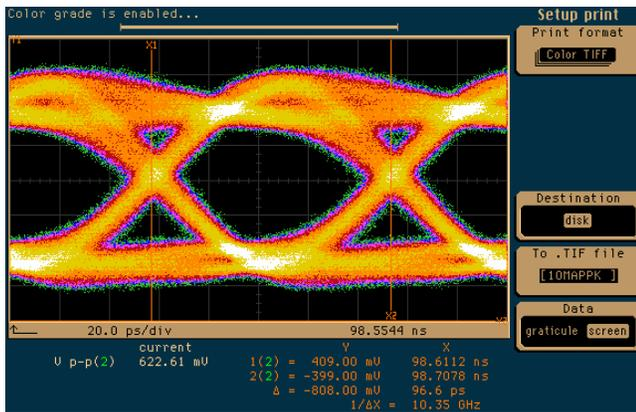
Fig.14: a) Measured 10.3Gb/s eye-diagram at the transmitter output with positive peaking only.
