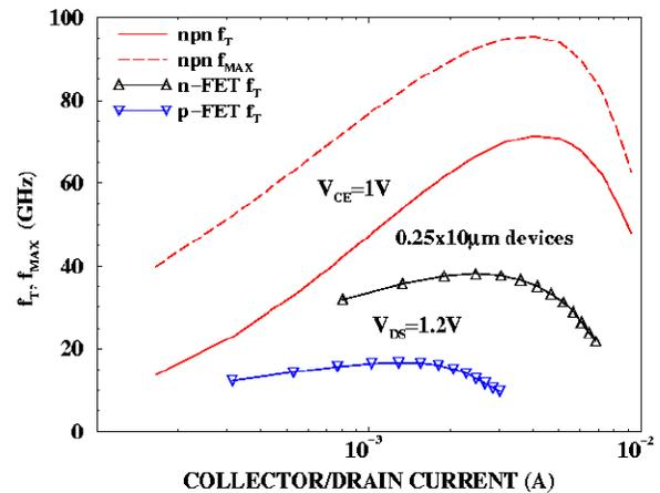
Fig.2: 0.25x10 $\mu$ m<sup>2</sup> npn,  $f_T$  and  $f_{MAX}$  characteristics as a function of the collector current. 0.25x10 $\mu$ m<sup>2</sup> n- and p-channel MOSFET  $f_T$  vs.  $I_{DS}$  characteristics are also shown.
