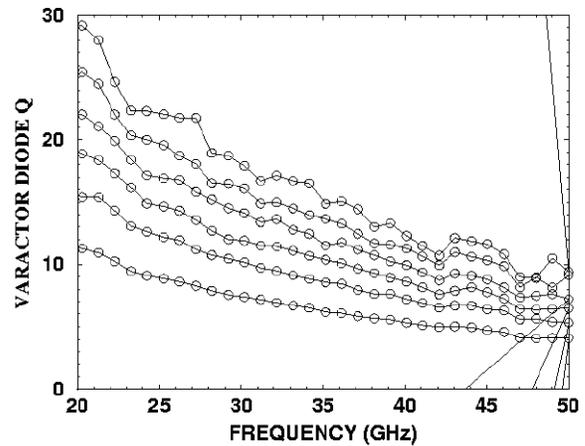
**Fig.7:** Measured quality factor of a 2x1.6 $\mu$ m x 20 $\mu$ m multi-stripe varactor diode in a SiGe HBT process as a function of frequency and varactor voltage between 0V and 5V.
