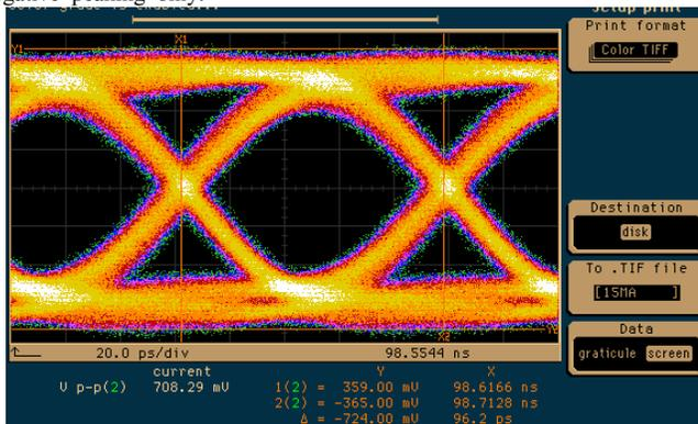
Fig.14: c) Measured 10.3Gb/s eye-diagram at the transmitter output with no peaking.
