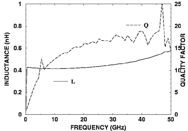
**Fig.6:** Measured inductance and quality factor of a 0.425nH octagonal inductor in a SiGe HBT process [15]
