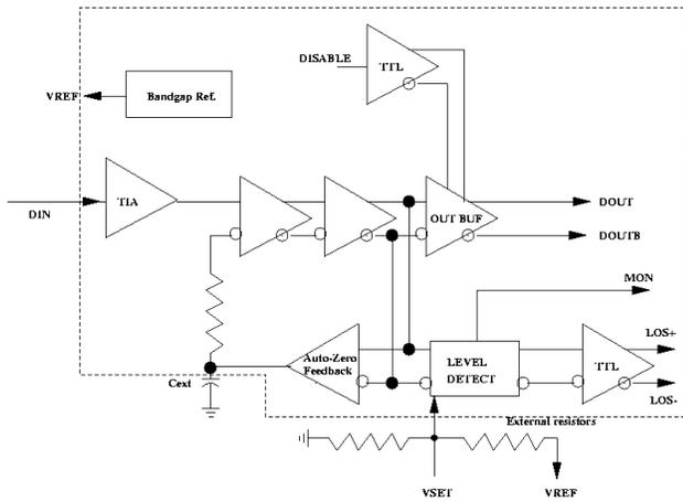
Fig.11: Block diagram of a 10.7Gb/s TIALA featuring linear monitor and LOS functions, as well as a dc-autozero feedback.
