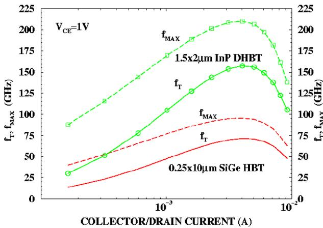
Fig.3:  $0.25 \times 10 \mu\text{m}^2$  SiGe HBT vs.  $1.5 \times 2 \mu\text{m}$  InP DHBT [11],  $f_T$  and  $f_{MAX}$  characteristics as a function of the collector current.
