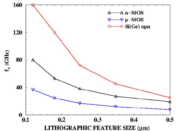
Fig.5: Scaling of Si CMOS and Si(Ge) npn devices as a function of feature size. The  $0.12 \mu\text{m}$  npn results are based on experimental data presented at the 2000 GaAs IC symposium with  $0.15 \mu\text{m}$  emitter widths [8].
