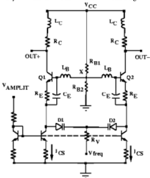
Fig.9: Schematic of a L-C-varactor VCO operating in the 20-30GHz range.
