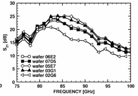
Fig. 12. LNA S<sub>21</sub> for technology splits.
