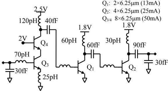
Fig. 3. 1.8V/2.5V, 77GHz, 3-stage power amplifier schematic.
