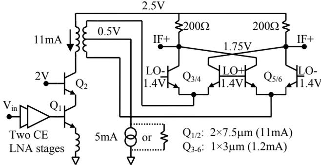
Fig. 4. Low-voltage double balanced mixer without RF pair.
