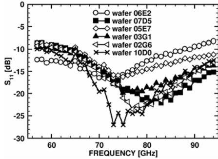
Fig. 16. PA Input return loss across technology splits.
