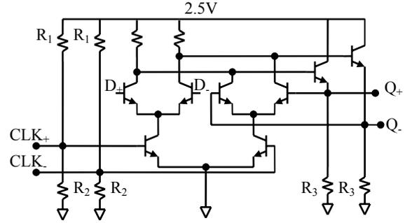
Fig. 5. Low-voltage D-latch used in 100GHz frequency divider.
