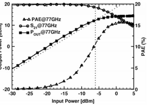
Fig. 15. PA S<sub>21</sub>, OP1dB, and P<sub>SAT</sub> at 77GHz
