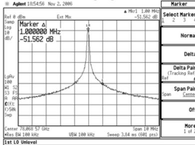
Fig. 7. VCO phase noise at 1MHz offset.
