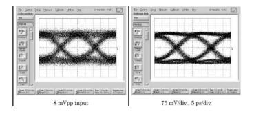
Fig. 21. Measured 43 Gb/s,  $2^{23} - 1$  input (8 mV<sub>PP</sub>) and output (320 mV<sub>PP</sub>) single-ended eye diagram of the TIALA mounted in a customer module as a limiting amplifier.
