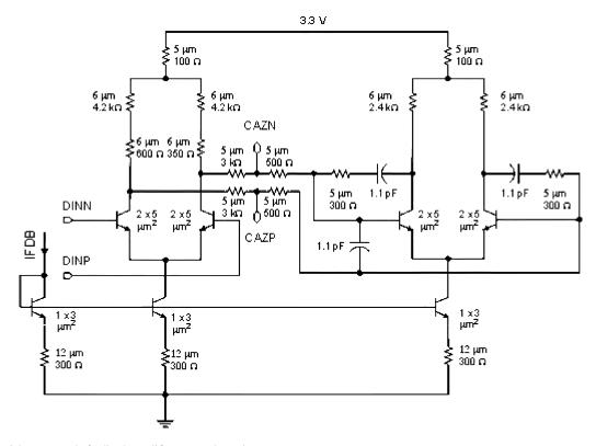
Fig. 9. Differential auto-zero dc feedback amplifier stage schematic.
