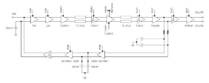
Fig. 1. Block diagram of the TIALA with single photodiode input. The unused TIA input is ac-coupled to ground in order to reduce noise. Emitter-follower stages are identified by a downward pointing arrow.
