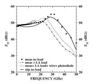
Fig. 14. Measured (symbols) and simulated (solid line)  $Z_{21}$  of the unloaded TIA on its own. Simulation results based on the measured unloaded TIA S-parameters and illustrating the impact of the estimated loading due to the LA (dotted-dashed line) and the impact of the photodiode capacitance and bondwire inductance (dotted line) are also included. The input impedance of the LA stage was approximated by a series connection of a 20- $\Omega$  resistance and an 80-fF capacitance.
