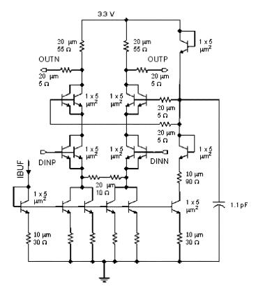
Fig. 8. Differential output stage schematic.
