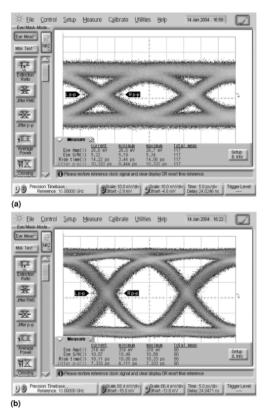
Fig. 19. On-wafer measured 43 Gb/s, single-ended input (a) and output (b) eye diagram corresponding to a 420  $\mu$ A<sub>pp</sub> input with  $2^{31} - 1$  PRBS.
