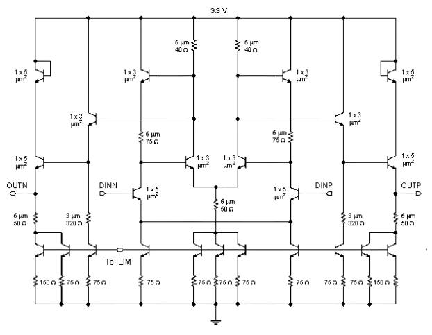
Fig. 6. Differential LA stage schematic.
