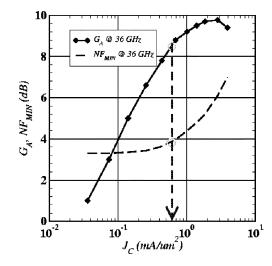
Fig. 3. Simulated  $NF_{\rm MIN}$  and  $G_a$  versus  $I_c$  characteristics of a  $1 \times 5 \,\mu {\rm m}^2$ InP HBT biased at  $V_{\rm CE} = 1$  V.
