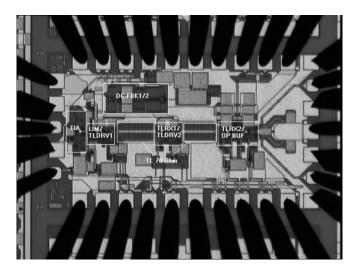
Fig. 10. Microphotograph of the TIALA with HF wafer probes.
