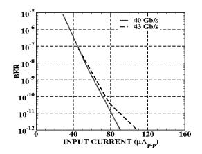
Fig. 15. Measured sensitivity with a  $2^{31} - 1$  PRBS.
