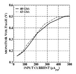
Fig. 16. Measured signal-level monitor output as a function of the  $2^{31} - 1$  PRBS signal level.
