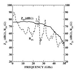
Fig. 13. On-wafer measured small-signal (with -65-dBm input signal) single-ended  $Z_{21}$  and input resistance of the TIALA.
