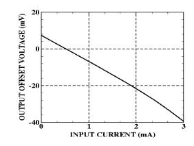
Fig. 11. Measured dc output offset as a function of dc input current.
