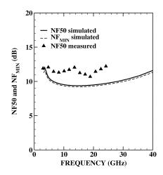
Fig. 5. Simulated and on-wafer measured  $50-\Omega$  noise figure, and simulated minimum noise figure of the TIALA. The bondwire inductance is not present in either simulations or measurements.
