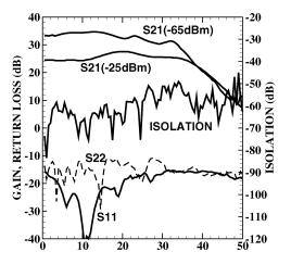
Fig. 12. On-wafer input/output return loss, isolation, small-signal (with -65 dBm input signal) and large-signal (-25 dBm input signal) single-ended TIALA power gain.
