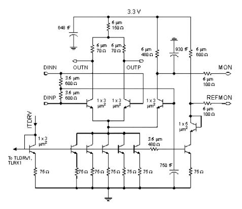
Fig. 7. Peak detector stage schematic and 70  $\Omega$  transmission line driver.
