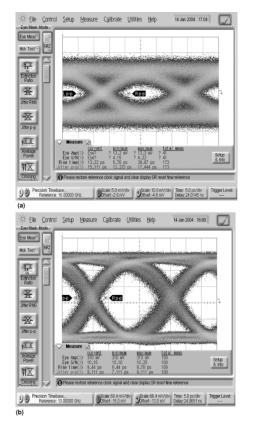
Fig. 20. On-wafer measured 43-Gb/s, single-ended input (a) and output (b) eye diagram corresponding to a 190  $\mu$ A<sub>pp</sub> input with 2<sup>31</sup> - 1 PRBS.
