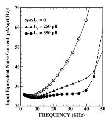
Fig. 4. Equivalent input noise current and gain simulation of the TIALA.
