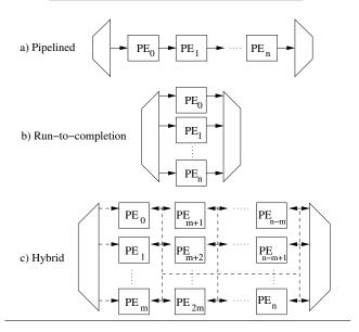
Figure 2: Parallelization models.
