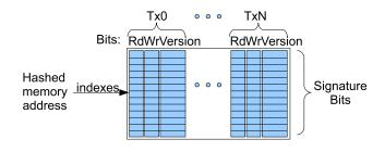
Figure 6: Signature table used to mark speculatively read and/or written for N hardware contexts. Version bits are used to distinguish between consecutive transactions on the same hardware context: a mismatch between this version and the context's transaction number indicates that the entry for that context is invalid.
