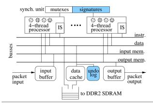
Figure 4: The NetThreads architecture, currently with two processors. NetTM supports TM by extending NetThreads, mainly with signatures and an undo-log.
