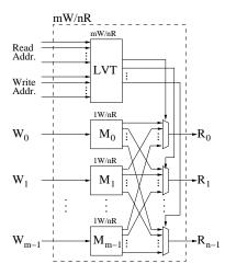
Figure 4: A generalized mW/nR memory implemented using a Live Value Table (LVT). Each write updates its own replicated memory bank (M) and updates its entry at the same address in the LVT. For each read, the LVT selects the memory bank that holds the most recently written value for the requested memory address.
