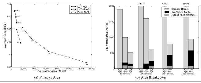
Figure 7: Speed and area for Pure-ALM, LVT-MLAB, and LVT-M9K implementations of a 2W/4R memory with an increasing number of memory elements.
