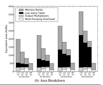
Figure 10: Speed and area for M9K-based 4W/8R multipumped memories: an LVT memory with multipumping factors of 1X (a 4W/8R memory with no multipumping), 2X (a 4W/4R memory with two internal cycles), and 4X (a 4W/2R memory with four internal cycles), and a pure multipumping memory (MP 3X).
