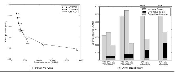
Figure 8: Speed and area for Pure-ALM, LVT-MLAB, and LVT-M9K implementations of a 4W/8R memory with an increasing number of memory elements.
