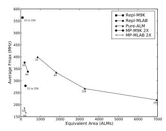
Figure 3: Comparison of the speed and area of various ALM, M9K, and MLAB implementations of 32-bit 1W/2R memories of varying depth (as indicated by the number at each data point). The prefix denotes the implementation technique: "Pure" for pure logic, "Repl" for replication, and "MP" for pure multipumping. The smallest possible M9K designs have a capacity of 256 elements, hence the two M9K designs are all overlapping. Placement/routing fail for MLAB designs of depth greater than 64.
