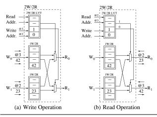
Figure 6: Example operation of a 2W/2R LVT-based multiported memory: during write operation,  $W_0$  writes 42 to address 3 and  $W_1$  writes 23 to address 2, and the LVT records for each address the bank that was last written; during read operation,  $R_0$  reads address 2 and  $R_1$  reads address 3, and the LVT selects the appropriate bank for each read address.
