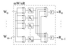
Figure 1: A multi-ported memory implemented with FPGA logic blocks, having D single-word storage locations (S), m write (W) ports, and n read (R) ports (encoded as mW/nR), and n temporary registers r. Only read and write data lines are shown (i.e., not address lines).
