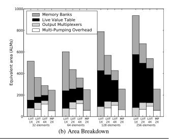
Figure 9: Speed and area for M9K-based 2W/4R multipumped memories: an LVT memory with multipumping factors of 1X (a 2W/4R memory with no multipumping), 2X (a 2W/2R memory with two internal cycles), and 4X (a 2W/1R memory with four internal cycles), and a pure multipumping memory (MP 2X).
