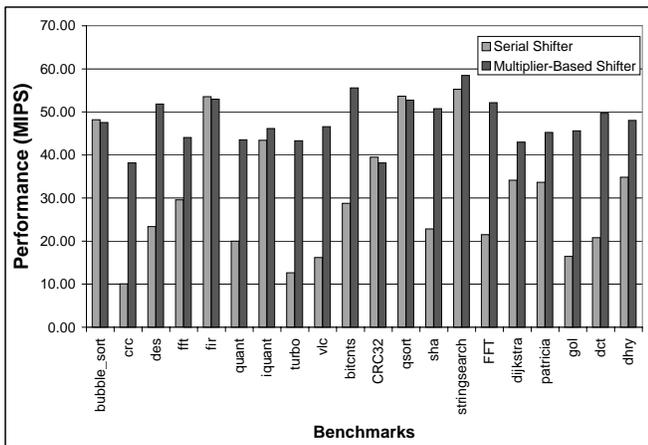
Fig. 3. Performance of a 3-stage pipelined processor with two different shifter implementations.
