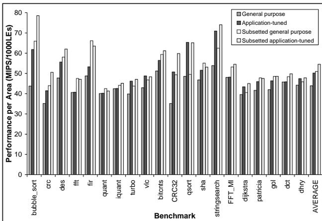
Fig. 14. Performance-per-area of tuning, subsetting, and their combination.
