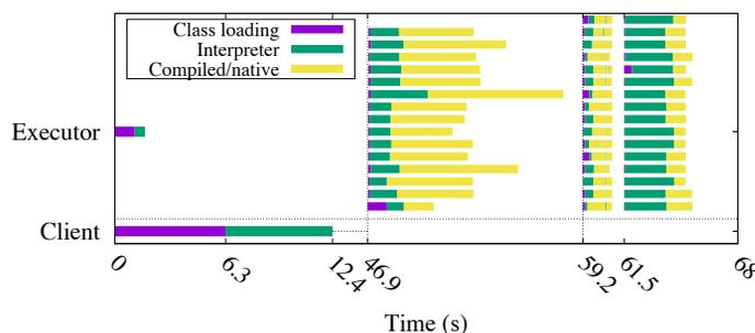
**Figure 6:** Breakdown of Spark's execution of query 13. It only shows one executor (there are a total of 10 executors, one per host). Each horizontal row represents a thread. The executor uses multiple threads to process this query. Each thread is used to process three tasks from three different stages.
