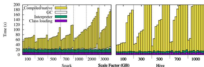
**Figure 5:** JVM overhead on BigBench. Overhead breakdown of queries from BigBench [3] across different scale factors. Only the 10 shortest queries from BigBench are analyzed because of our focus on latency-sensitive queries. The scale factor corresponds to the size of input data in GB. The queries are first grouped by scale factor and then ordered by runtime. Note that Hive has a larger query time compared to Spark.
